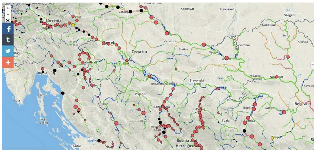
Picture 4: Hydropower plants in Sava basin: Existing (black), planned (red) and under construction (yellow). Riverwatch/EuroNatur 2012. http://balkanrivers.net/en/map
