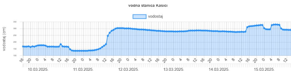
Figure 9: Records from the water level station at Kašići. The fluctuations observed on 15 March 2024 are of anthropogenic origin and are due to the operation of the Ulog power plant (source: https://www.fop.fhmzbih.gov.ba/ ).
